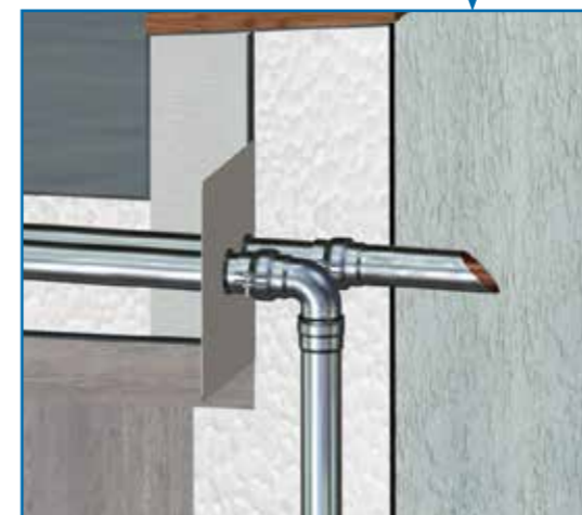
For the penetration through the vapor barrier of pipes that are lying next to each other
